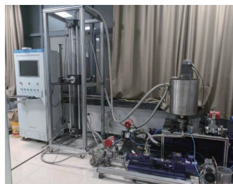
图 2 煤层气井煤粉动态运移沉降测试系统 Fig. 2 Dynamic migration and settlement testing system for coal powder in coalbed methane wells
