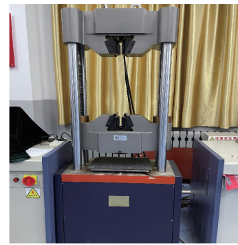
图 1 YNS300 微机控制电液伺服万能试验机 Fig. 1 YNS300 microcomputer-controlled electro-hydraulic servo universal testing machine
